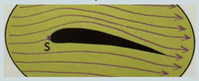
**Bernoulli's Principle** states that as the speed of a fluid (like air) increases, its pressure decreases.
