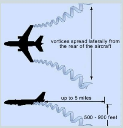
Wake turbulence is the disturbed, rotating air left behind by an aircraft as it generates lift.
